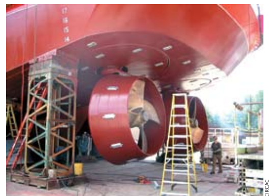
The tug Vigilant's twin z-drive engines can rotate 360 degrees to provide optimal escort and assist capabilities, and are rated up to a maximum of 6,772 horsepower.
